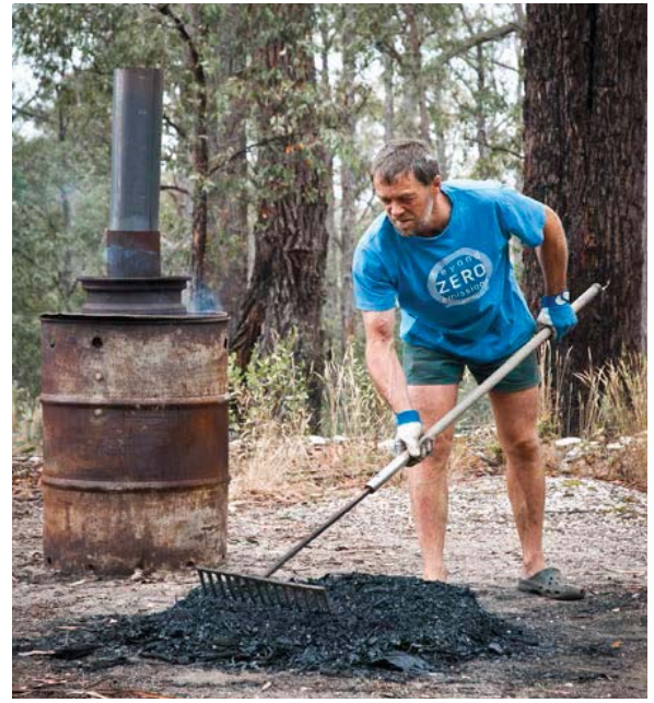
↑ Inspecting the previous charred batch, while the next one is being fired. Notice that minimal smoke is being emitted.
